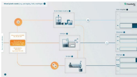
With the CCPE recycling cascade for plastic waste, consisting of a combination of three Fraunhofer technologies, high-quality plastic recyclates can be produced with an optimised product yield. © Fraunhofer CCPE
